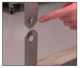
Figure 1-4. Applicator frame connector.
