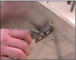
Figure 1-6. Drain tray hook.
