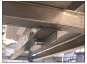
Figure 1-7. Bucket support fasteners.
