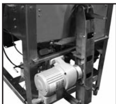
New energy efficient oil-free drive system.
