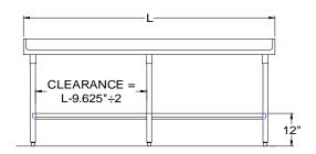
All units ship unassembled for reduced shipping cost. Units 7 ft. and larger are furnished with six legs. All dimensions are typical. Tolerance +/- .500".
