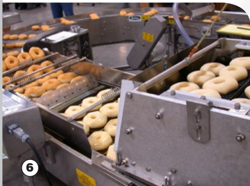
Above: 4– Standard Mark VI system 5– Mark VI system with automatic Proofer and Glazer 6– Automatic proofer with Deep Mark VI fryer in Automatic system
